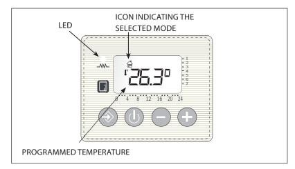
There is an LED light on the control panel: when the system is in heating mode and the room temperature has not yet reached the desired temperature programmed by the user, the LED is RED. Once the room reaches the programmed temperature, the LED turns GREEN.
