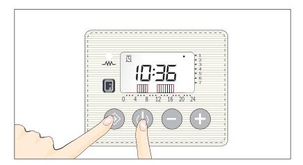
A dot will blink on the screen next to the days of the week (1-7). The current day can be selected using the plus or minus key. Use the 'mode' key to confirm the selection.
